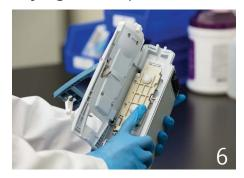
Fully inspect the instrument during each cleaning. Look for any visible external damage, such as a cracked or broken door, handle or latch. Open the door of each pump module, and inspect the platen and hinge for cracks or other damage.
