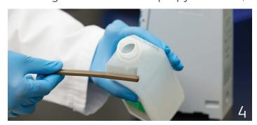
Remove IUI connector covers. Apply 70% IPA directly to the dedicated IUI cleaning brush. To prevent cross-contamination, do not dip the brush into the IPA.
