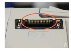
Inspect the IUI connectors on each BD Alaris™ PC Unit and module prior to use. Replace any IUI connector with surface contaminants, blue or green deposits, damaged contacts, ribs or cracks.
