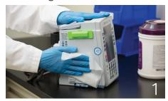
Make sure the instrument is upright, turned off and the power cord is unplugged. Attach strongly recommended IUI connector covers. Wipe all exposed device surfaces **EXCEPT** the inter-unit interface (IUI) connectors.
